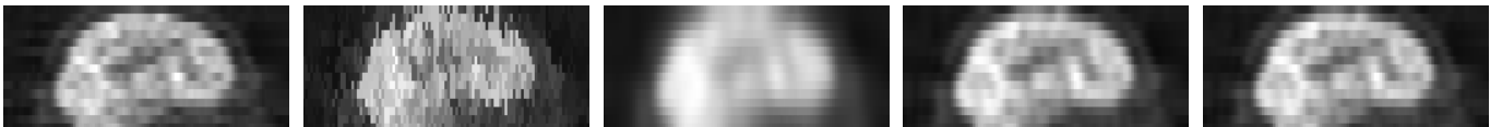
Figure 4: Visual impression of the errors resulting from the rotation experiment carried out on a sagittal slice of a PET dataset (left), when using (from second left to right) nearest-neighbor (zeroth-degree spline) interpolation, linear (first-degree spline) interpolation, and cubic and quintic spline interpolation, respectively. Note that the displayed images are scaled so as to visually correct for the voxel anisotropy.
